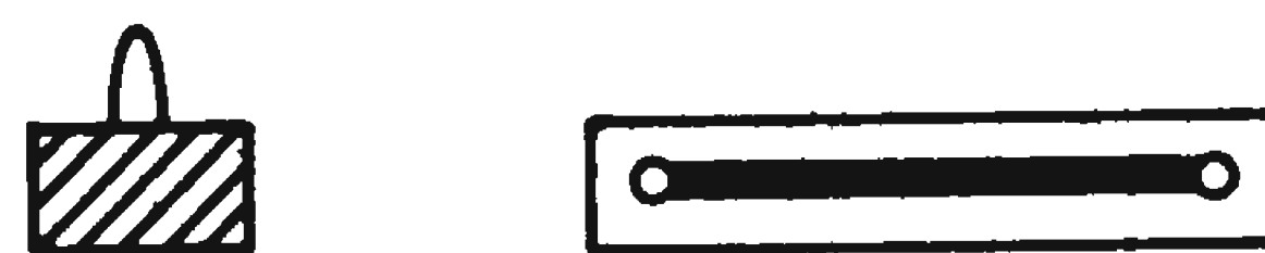
Fig. 1. Wire printed on a card can be plugged into printed-circuit card to alter circuit configuration.
